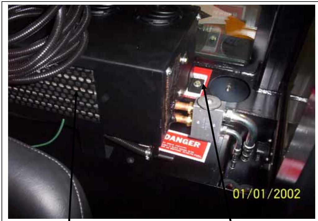
Evaporator mounted in place.
