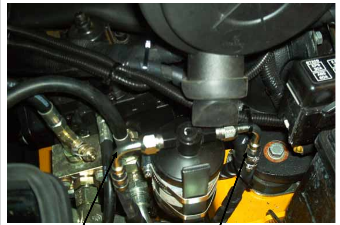
#6 hose out to expansion valve.
