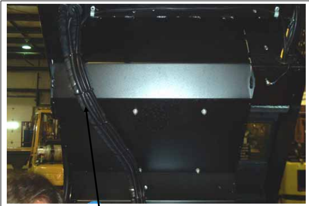
Hoses and wiring running from cab to engine compartment.
