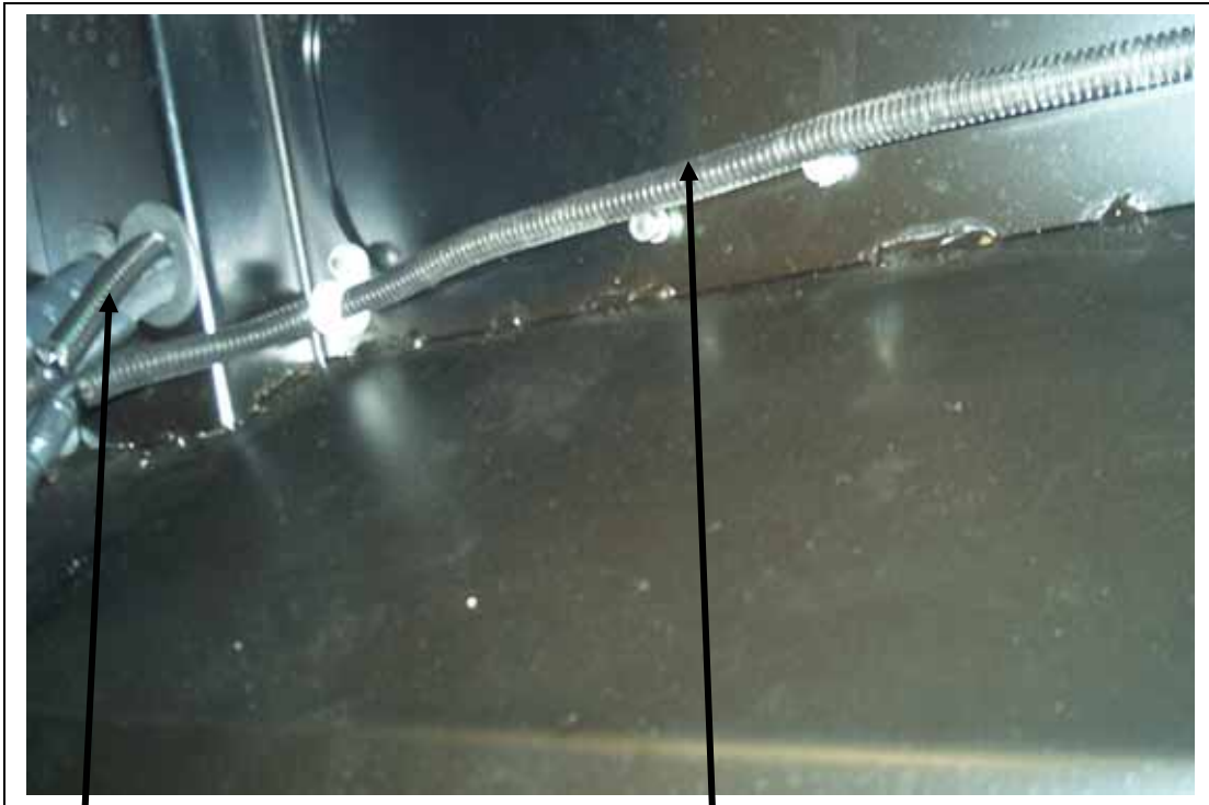
14ga white clutch wire out with hoses to engine compartment.
