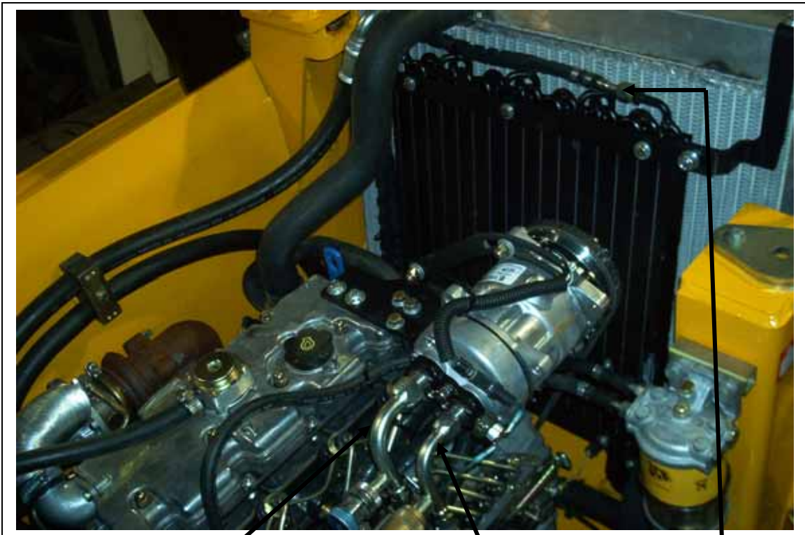
1/2" hose to the expansion valve
